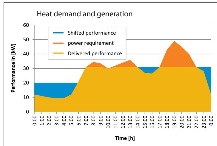
This daily load curve shows a typical output requirement distributed over one day. To cover the highest peaks, you need to install a heat generator that can cover the output peaks.
